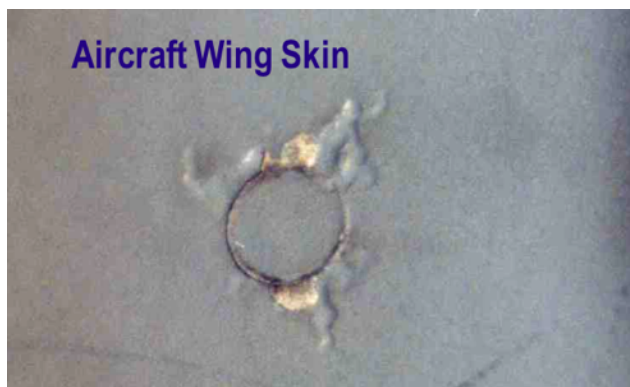
Figure 14. Filiform corrosion propagating from cracked paint around a fastener head on the skin of an aircraft wing.
